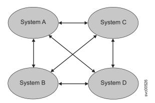
Figure 22. Systems in a fully connected mesh configuration. Every system has a partnership to each of the three other systems.
