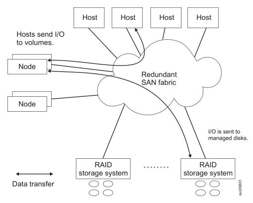
Figure 2. Data flow in a SAN Volume Controller system
