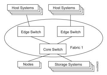
Figure 33. SAN configuration with a medium-sized fabric
