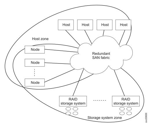
Figure 1. SAN Volume Controller system in a fabric
