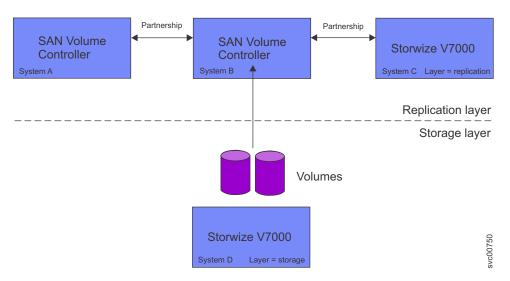
Figure 25. Example configuration for replication between SAN Volume Controller and a Storwize V7000 system
