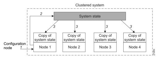
Figure 6. Clustered system, nodes, and system state
