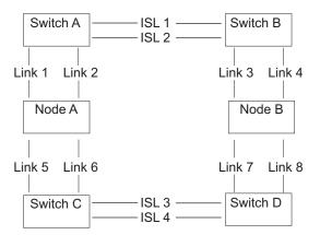
Figure 31. Fabric with ISL in a redundant configuration
