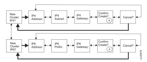
Figure 40. New Cluster IP4? and New Cluster IP6? options on the front-panel display
