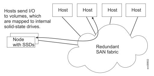
Figure 3. SAN Volume Controller nodes with internal SSDs
